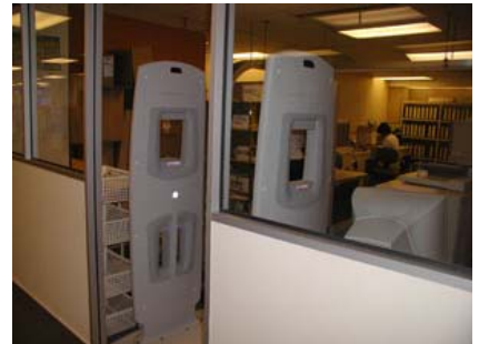
The EAS Gantry prevents unauthorized items from being taken out of the library.
